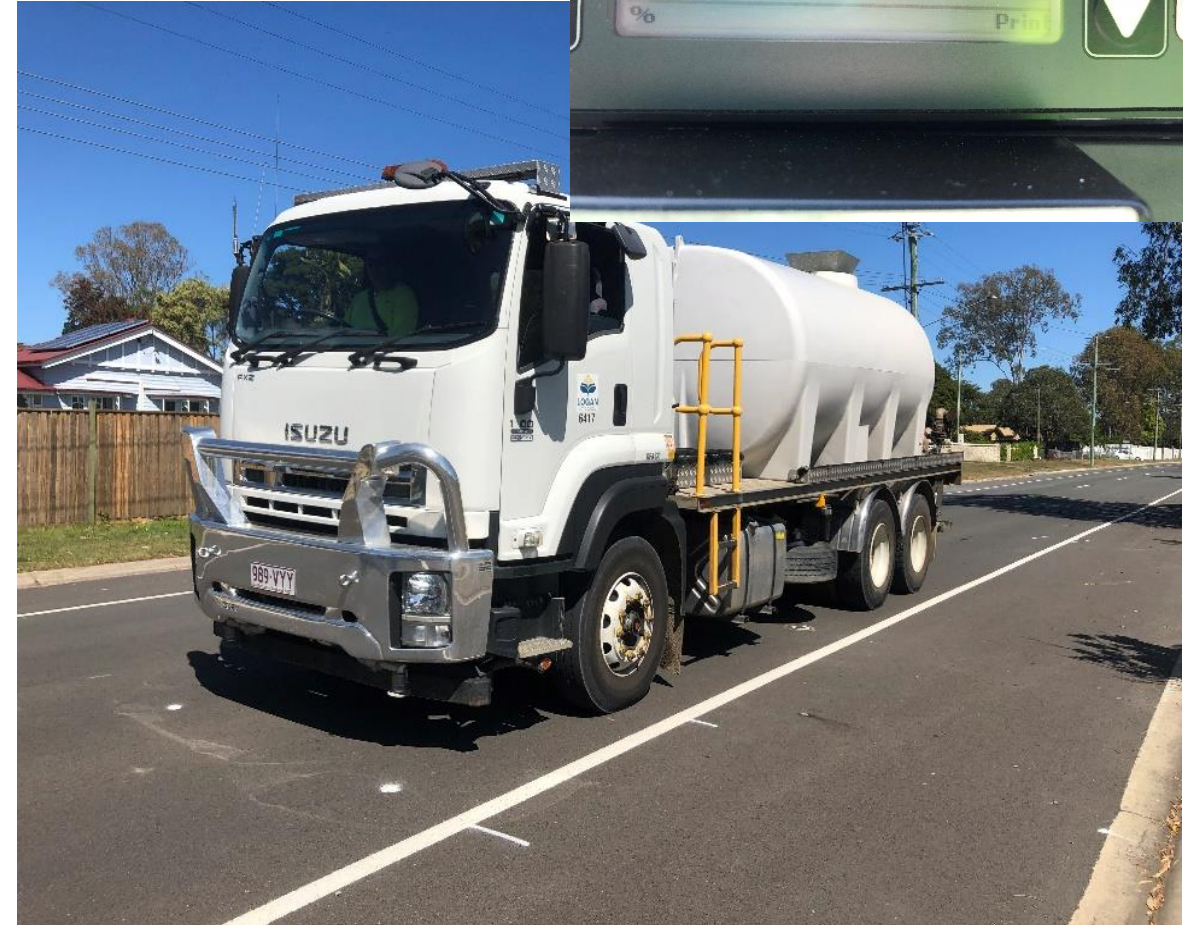
Front axel tyre on each pressure cell location for 5 min (6.9 T axel load)
