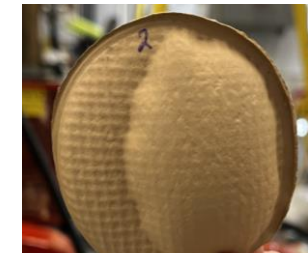
Chlorosulfonated polyethylene (CSPE), no major changes on surface
