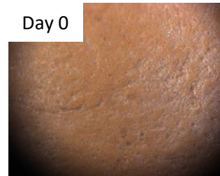
Chlorosulfonated polyethylene (CSPE), no major changes on surface
