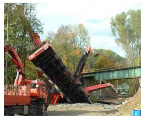
Rotational failure at the edge of platform, Brunei, Asia
