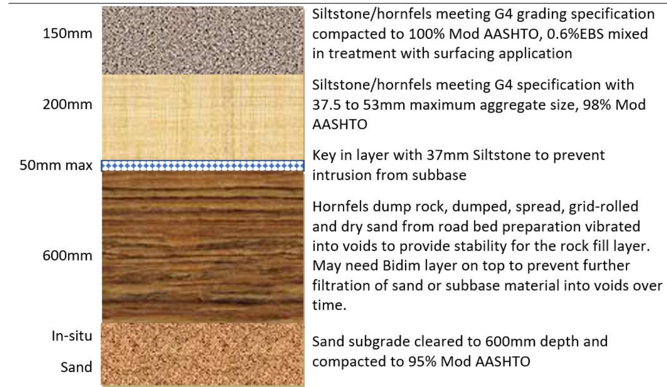
Original design – 600mm rockfill
