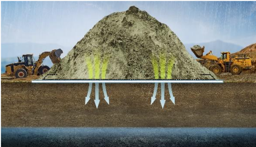
Short term storage of contaminated soils (laydown pads)
