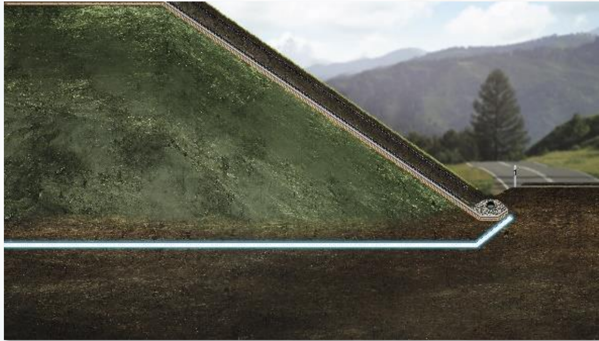
Permanent closure (capping) of a contaminated spoil
